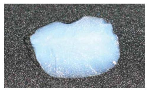
A piece of Aerogel made by NASA's Jet Propulsion Laboratory for catching stardust. At 99.8% air, this is the lightest solid in the world and is blue for the same reason that the sky is blue.
